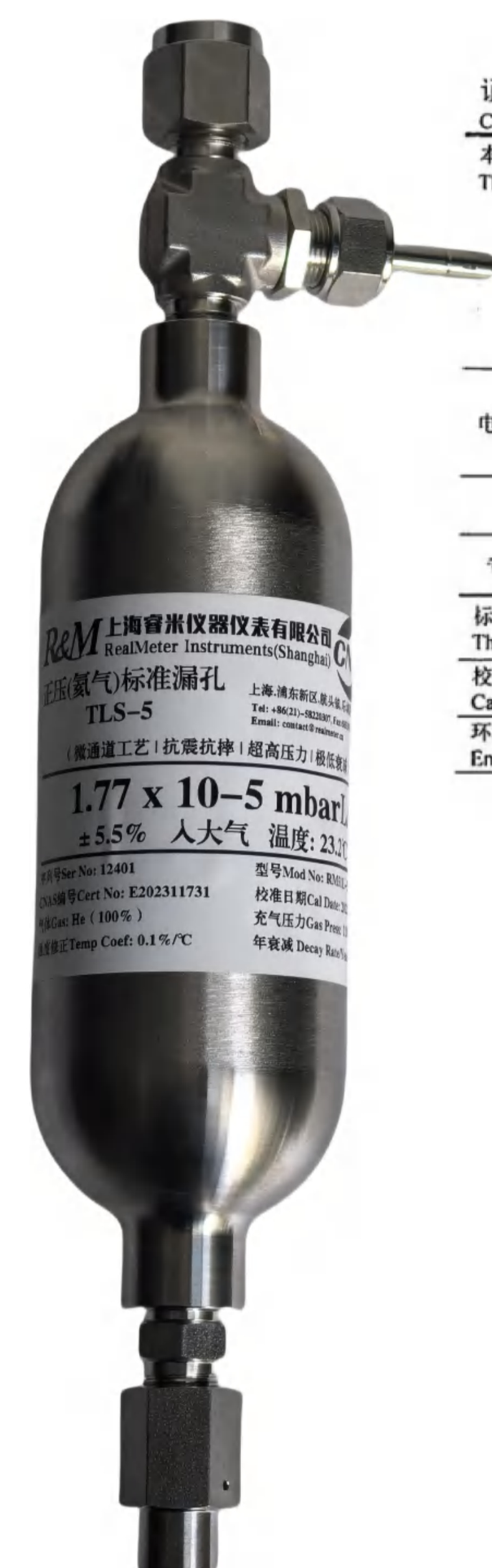
He有源正压漏孔 1.77E-5mbar.L/sec
