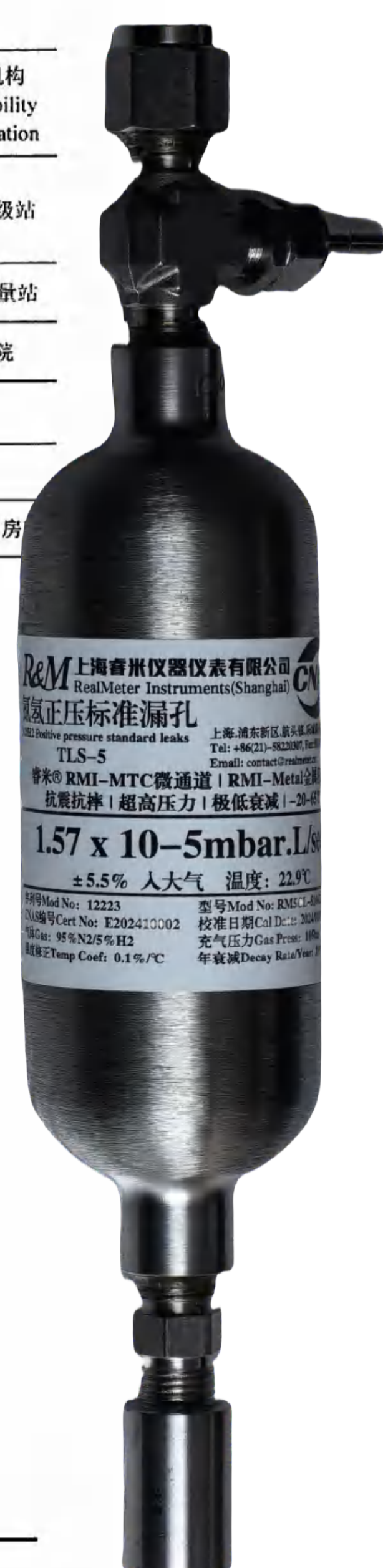
He有源正压漏孔 1.57E-5mbar.L/sec
