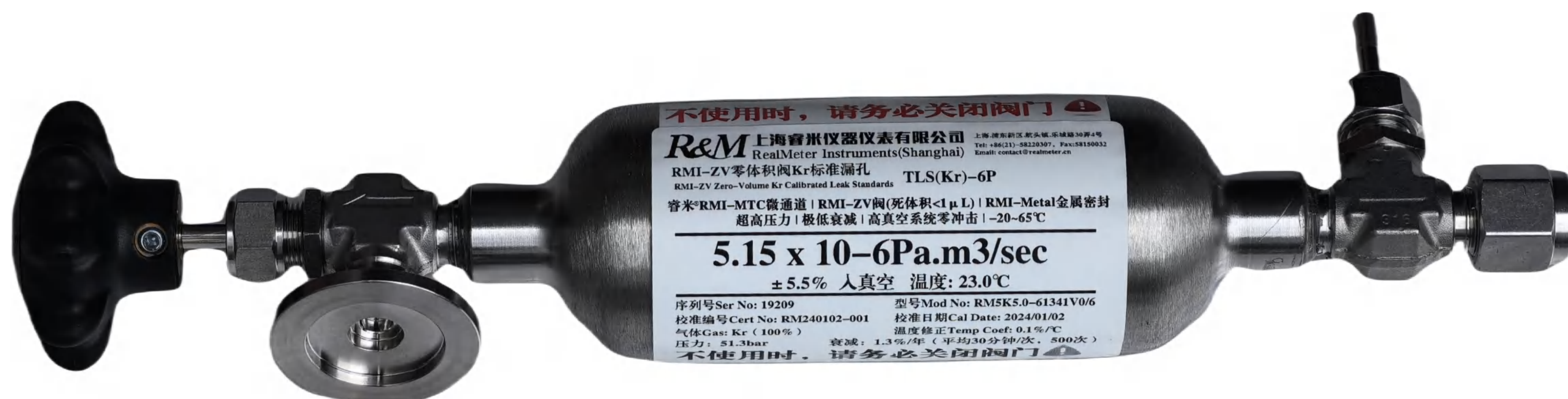
实物照片: 氪气Kr标准漏孔, 5.15x10 -6 pa.m 3 /sec, KF25, , RMI-MZV阀
