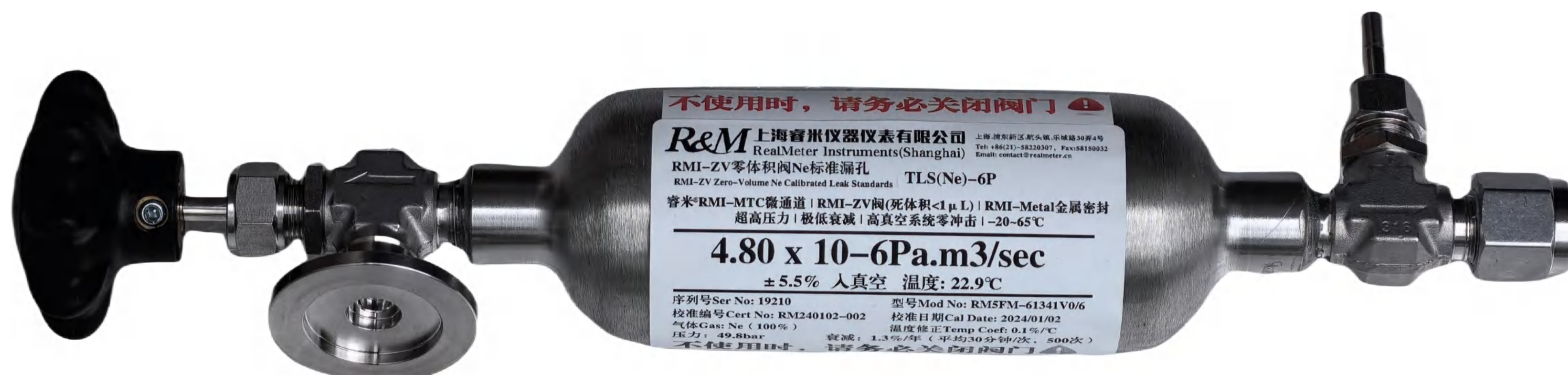
实物照片: 氖气Ne标准漏孔, 4.80x10 -6 pa.m 3 /sec, KF25, RMI-MZV阀
